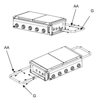
10. With the help of an assistant, align the grill body to the cart as shown below, then lock the four latches, securing the firebox to the cart.
