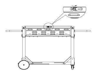
12. Unfold side shelf, left & right and wind shield and place the tabs of the side wind shields into the small openings securing the windshield. Remark: The lighting stick is preassembled on the cart leg
