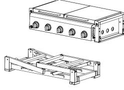
7. Attach the wheel axle (F) through the cart legs, as shown below picture, then attach the two wheels (E) with two M12 nuts (CC), and attach two wheel caps (D) with two 1/4-in. x 12mm round head screws (DD) and two1/4-in flat washers (EE) at the end of the wheel axle (F).
